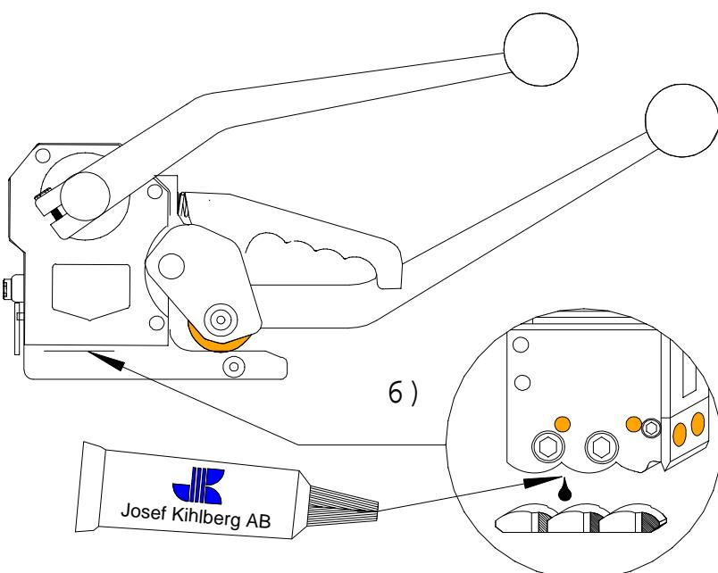
**E** Apply a little shearing oil (Nr 189323) to the surface of the punches (6) and then operate the strapper a few times without any strapping.
